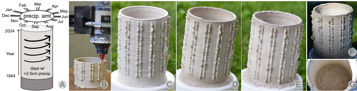
Figure 1: This work explores the design and sustainability of 3D printed clay physicalizations. Rain Gauge is a clay data physicalization depicting monthly precipitation data from 1944-2024. A. monthly precipitation encoded as line length; B. clay 3D printing process; C-E. progression as the Rain Gauge receives rainfall; F-G. lasting rainfall effects.
